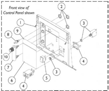
NOTE: There are 2 styles of #10 - flowmeter knobs. These knobs are NOT interchangeable. Refer to the photos below.
