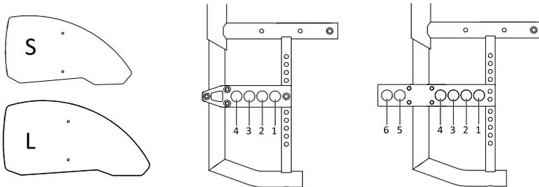
Clothes guard with respect to the position of the rear wheels with standard adapter plate (Pos. 1 to 4) or rear wheel extension (Pos. 5 and 6)
