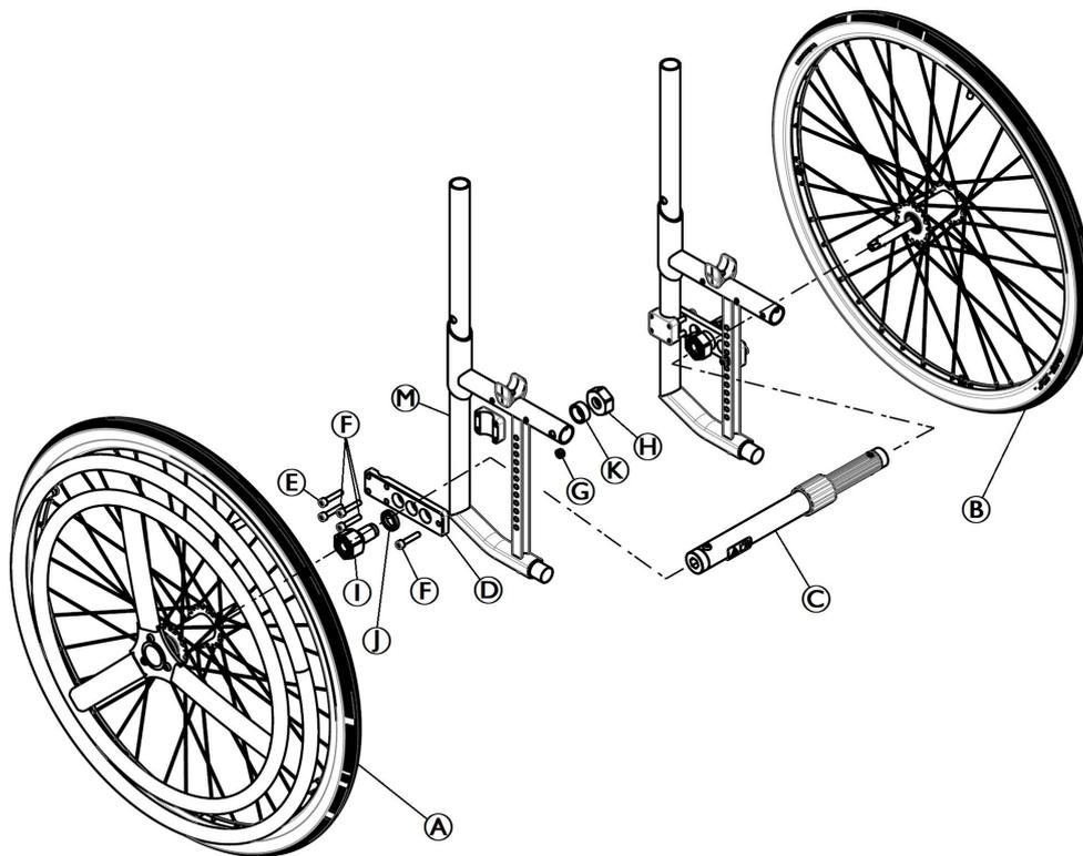
1. Install the adapter plate **D** to the frame **M** using bolt **E** and bolts **F** with washer and nut **G**.
