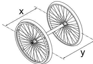
3. In accordance with the table, turn the adapter sleeves so that the distance between the rear wheels is the same at the front and the back ( $x = y$ ) – measured at the height of the center of the axle.
