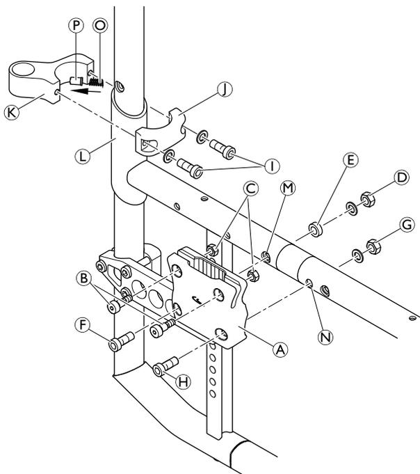
**Installing/Removing the Armrest, T-Armrest Pad and Cover**
